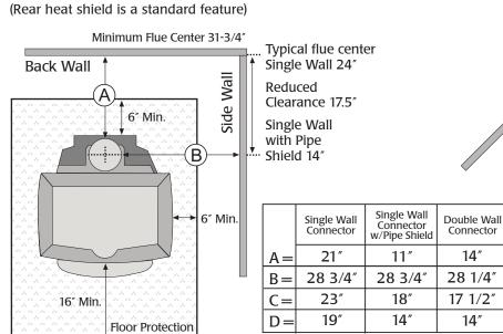
Measure front hearth pad clearances from the face of the stove (door opening). Measure rear hearth pad clearances from the back of the heat shield.
